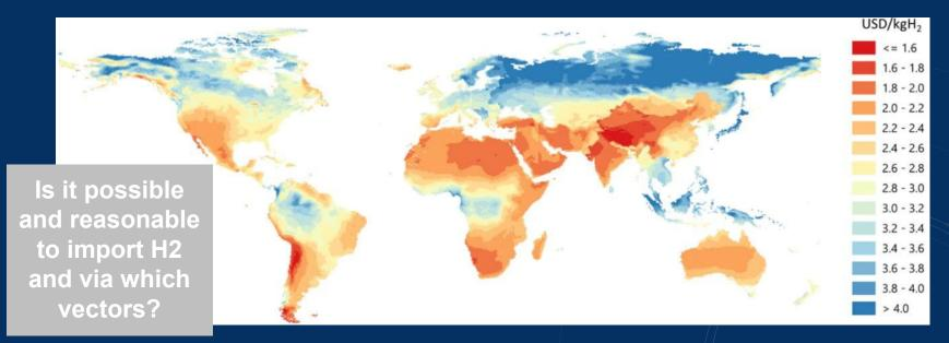
**Source:** The Future of Hydrogen, Report by IEA, June 2019 Assumptions: ELY efficiency 74%, CAPEX 450 US\$/kW (ELY), 400 - 1,000 US\$/kW (PV), 900 - 2,500 US\$/kW (onshore wind) Hybrid plants combining wind and PV
