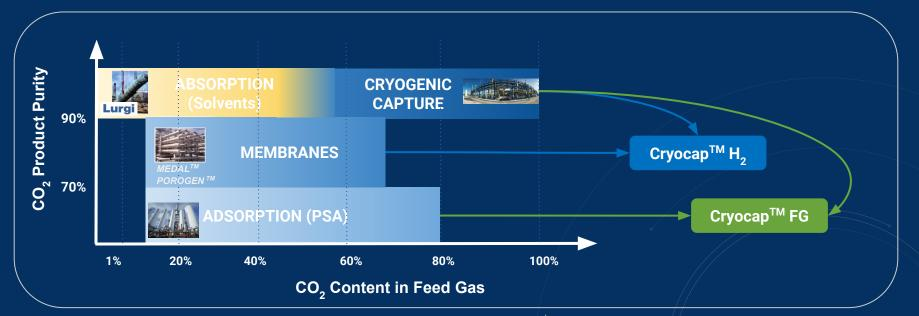
Absorption: The most suitable solution for low concentrated feed gas
