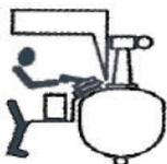
A Local Exhaust Ventilation (LEV) system is used to contain the contaminants within a defined area and draw airborne contaminants away from the operators' breathing zone. This can involve either:
